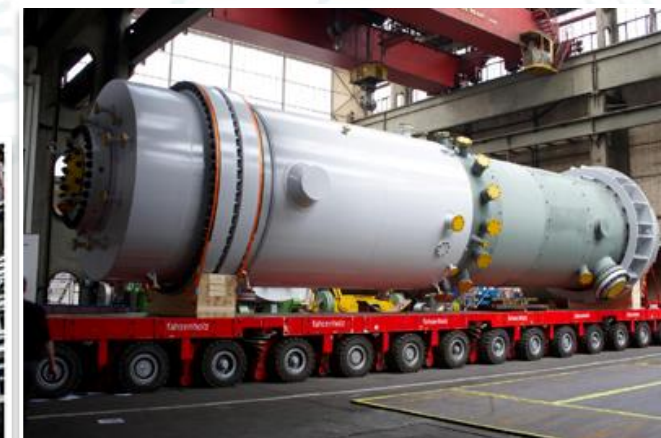
SNG-plant, CPI Xinjiang Energy Co. Ltd, Yili City Xingjiang, China, 8 x 500 MW Siemens SFG-500 coal-gasifier, commissioning 2014
